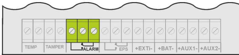
Fig. 9. Technical output ALARM.
