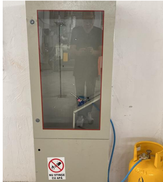
Flame test cabinet according standard
